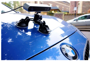
Fig. 10. Experimental set-up for acquiring stereo road images.
